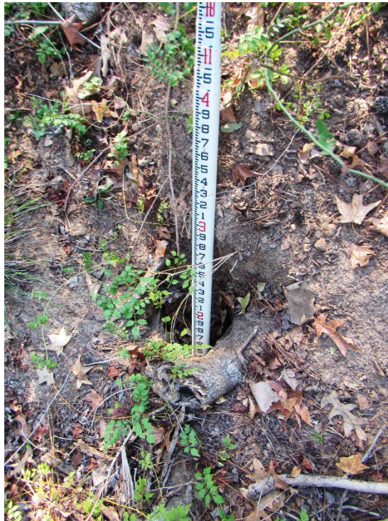
Photo 10. View of a burrow along the downstream slope, about 1.7-feet deep, near the mid-left end of the dam. Note the dead tree roots adjacent to the burrow.
